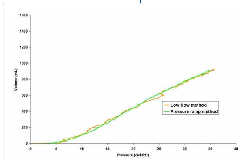
Figure 1: Typical pressure/volume curves obtained with the Low Constant Flow (orange) and the Linear Pressure Ramp (green) methods in a patient with restrictive lung disease.
