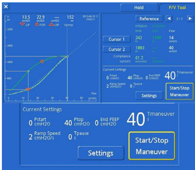
Figure 1: Setting of the pressure-volume curve using P/V Tool Pro
