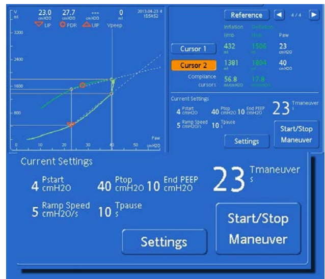
Figure 17: Settings for a recruitment maneuver with the PV Tool using a fast pressure increase (ramp speed at 5 cmH2O/s), a pause of 10 s at high pressure, and higher PEEP after the recruitment maneuver
