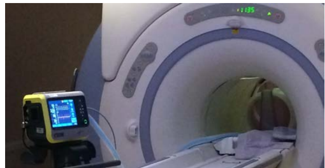
Figure 2: Ventilator positioning for low-load test with 3T scanner
