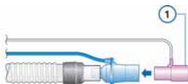
Figure 2-13 Attaching the CO2 sensor (1) to the airway
