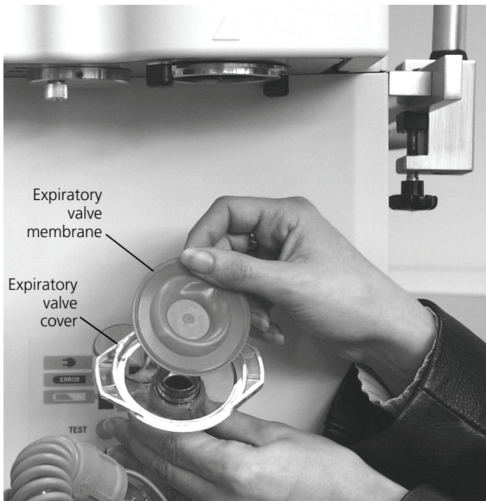
Figure 2-9. Installing the expiratory valve membrane
