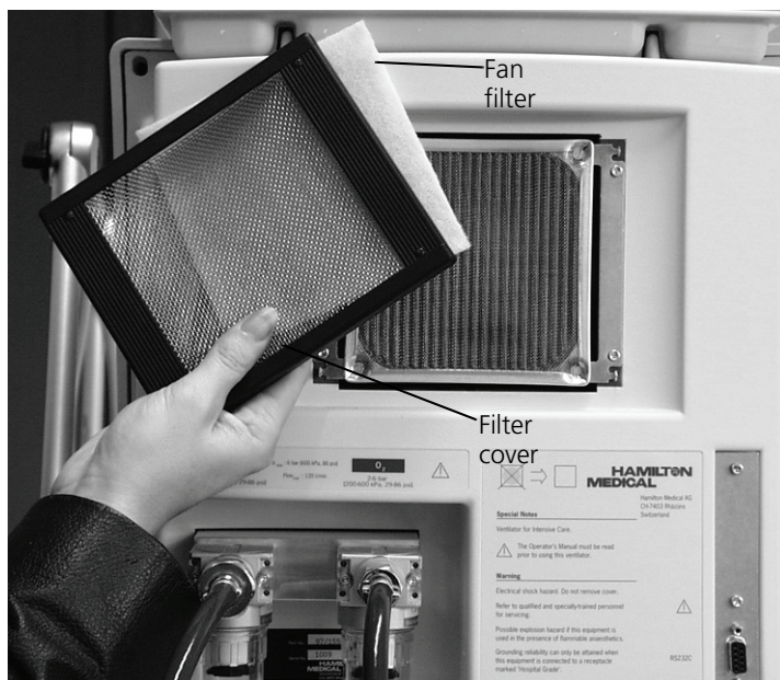
Figure 10-1. Removing the fan filter
