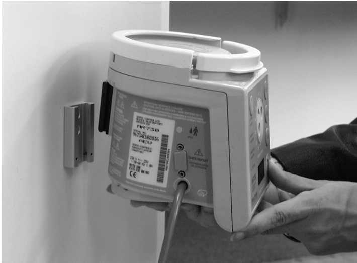
Figure 2-3. Installing the humidifier
