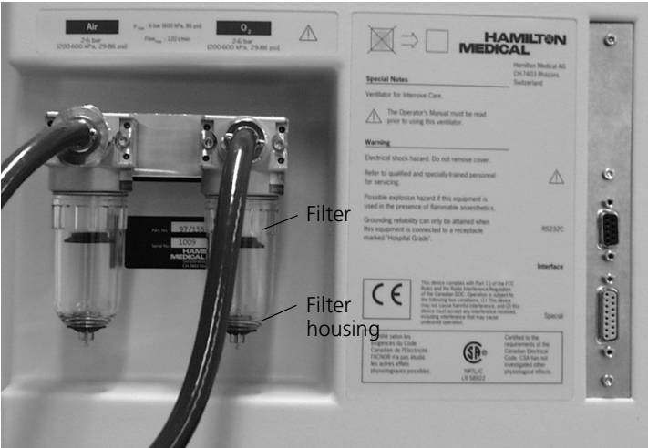
Figure 10-2. Replacing a gas supply filter
