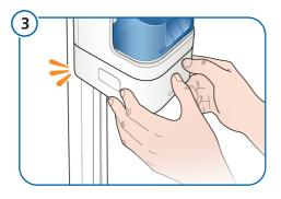
An audible click indicates the battery is locked in place.
