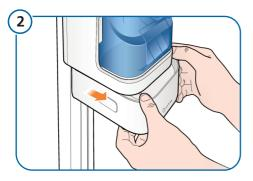
Carefully slide the battery forward.
