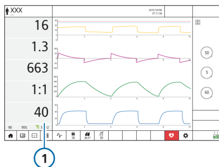
Figure 2-18. Main display showing PetCO2 as MMP (1)
