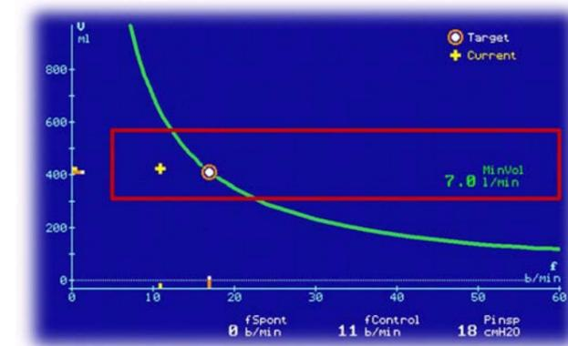
The special ASV window, showing the (red) frame of maximum safety, the (green) curve indicating the range of all breath frequency/tidal volume values for the set minute volume, the (circle) Target marker indicating the frequency and tidal volume offering the lowest work of breathing, and the (cross) Current marker, showing the current status.
