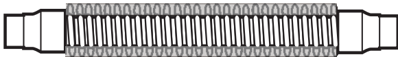
Figure 2. Compressible volume. The gray area represents the additional volume attributable to patient circuit compliance. Compliance compensation equations subtract this volume to produce the calculated VTE.
